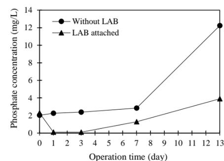
Even though the **LAB** is attached to the BC, they are **effective** at removing phosphate from the aqueous solution. **LAB-attached BC** can be an **absorbent for phosphate removal**.
